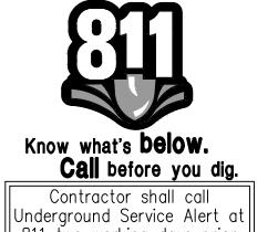
Contractor shall call Underground Service Alert at 811 two working days prior to excavation
